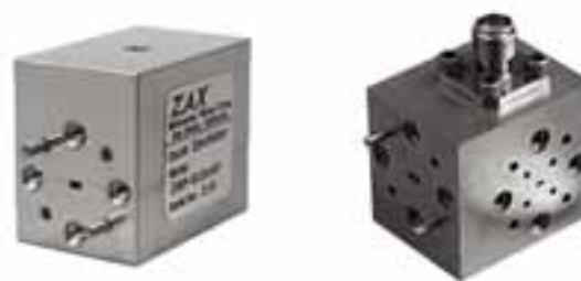
Figure 2. ZAX fixed frequency Gunn diode oscillator operating near 89 GHz with WR-10 waveguide output (left) and sub-millimeter-wave mixer with WR-5 RF input, WR-10 LO input and SMA IF output.
