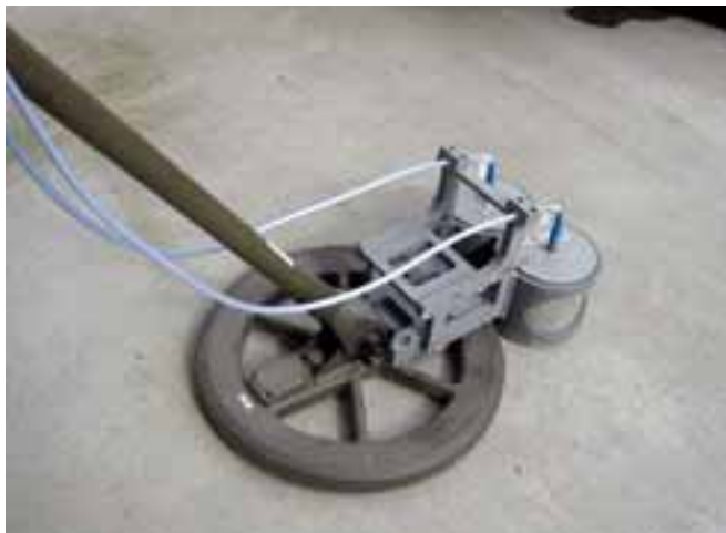
Figure 5. GPR antennas and metal detector sensor of ALIS.
