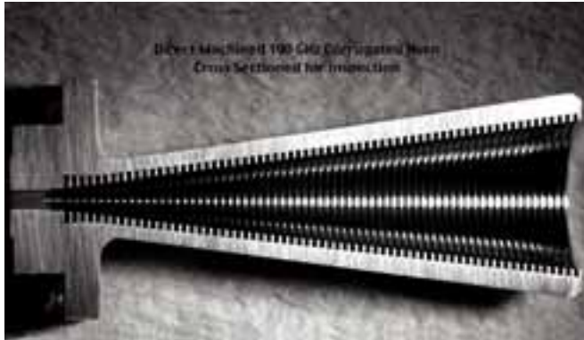
Figure 3. Cross-section of a 190-GHz corrugated horn antenna manufactured by using direct machining. Note the ratio of the largest to smallest radius at the throat of the horn must allow clearance for removal of cutting tools.
