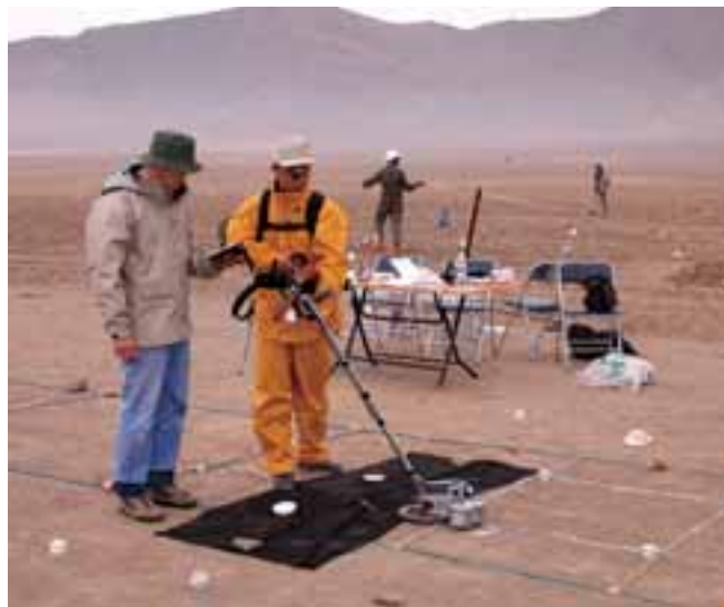
Figure 4. ALIS under test at CDS test site, Afghanistan.
