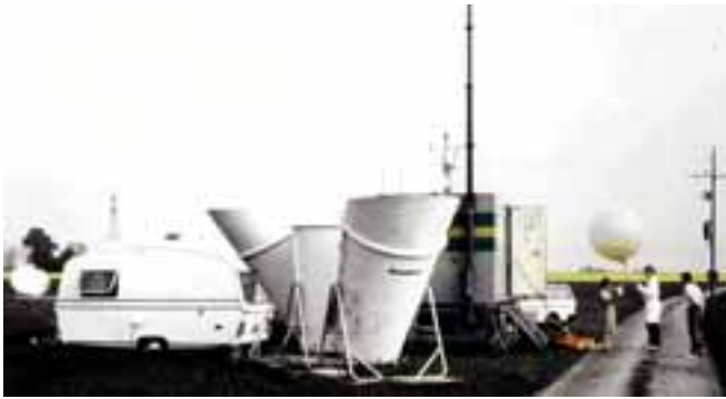
Fig. 2. Atmospheric observations in 1984 using temperature profiling radiometer (in caravan) as part of a field experiment for investigating the atmospheric circulation in the neighborhood of a nuclear power station.
