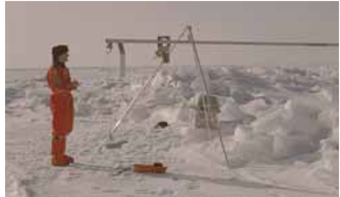
Fig. 3 In situ measurement of sea ice roughness during the Baltic campaign of 1994 by means of laser device.
