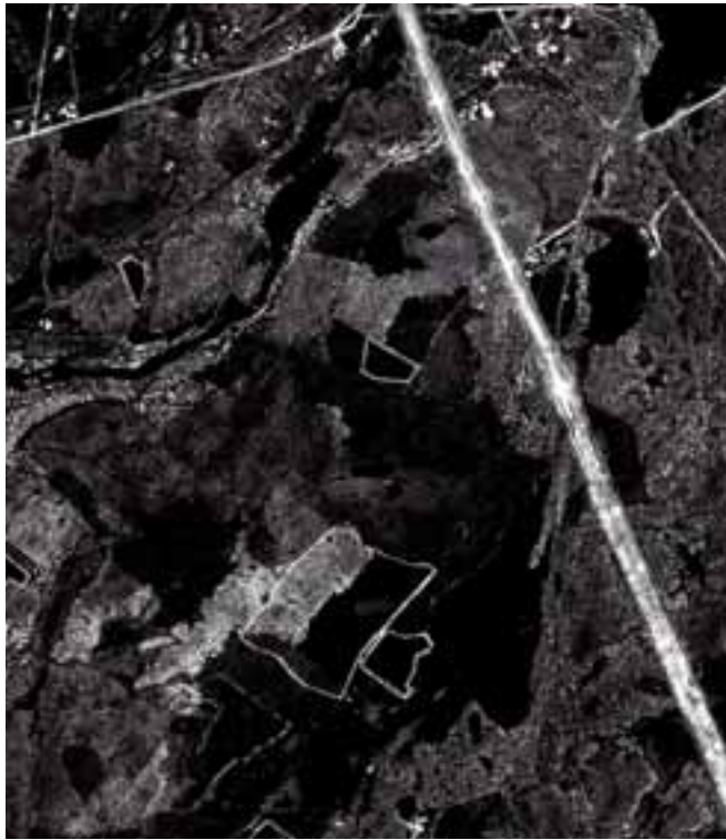
Fig. 5. CARABAS image of a mixed forest in Southern Sweden, produced by combining images from multiple flight directions. Buildings and linear metallic structures (fences, overhead cables, etc.) appear very bright. Grey tones in forested areas are related to biomass, varying from unforested areas (black) to dense forest (aboveground biomass ~400 tons/ha). The image covers an area of 1.25 km by 1.5 km.
