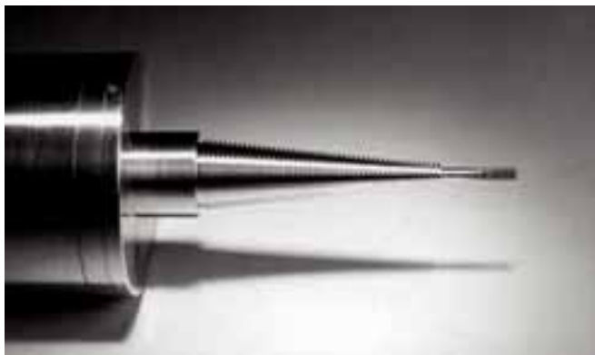
Figure 4. Model of the internal geometry of the corrugated feedhorn representing the first step of the electroforming process. Creating the geometry 'inside-out' allows designs to be created by the electroforming process that can not be manufactured by direct machining.
